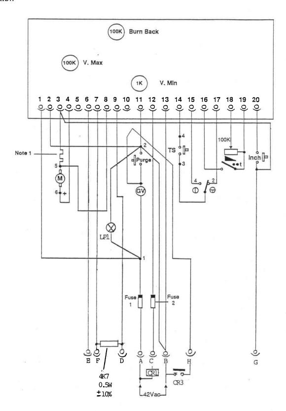
Note 1: "IR" compensation resistor = 500mm 0.5mm<sup>2</sup> copper
